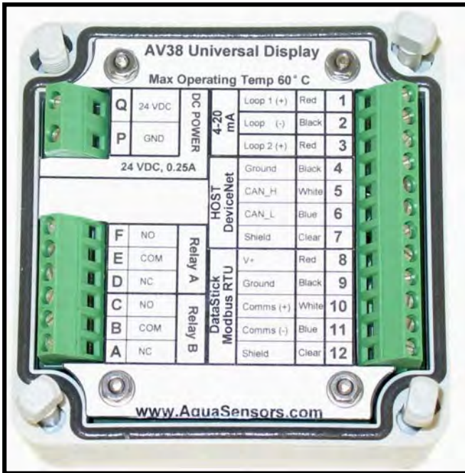
DC-powered AV38 with DeviceNet host comms wiring
