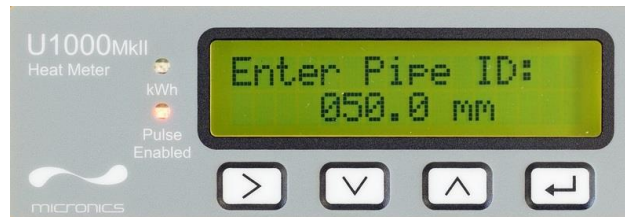
Figure 11 Enter Pipe ID Screen (Metric)
